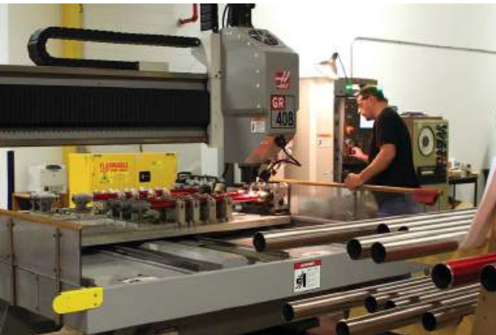
The CNC milling machine can machine up to six tubes at once.
